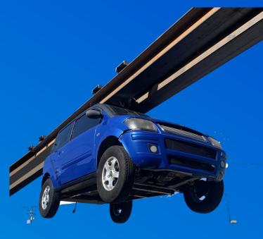
GoBFree cars and trucks drive like regular vehicles to local destinations but for longer distances and commuter travel they attach to an overhead rail. As drivers relax, work, or even sleep the batteries are automatically charged.
